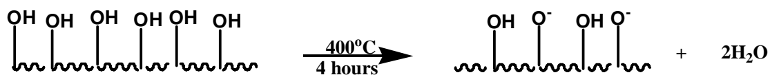
Fig 2.1.1.4d Optimum temperature and time for the activation of gamma alumina using “thermal condition”
